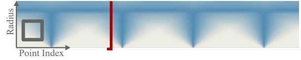
Figure 3: The multi-scale feature image (MSFI) illustrates the geometric measures by mixing the base colors; pixel columns (vertically) denote a single measure graph at a specific location, for varying radii. The red line marks the geometric measures for the point on the square in Figure 2.
