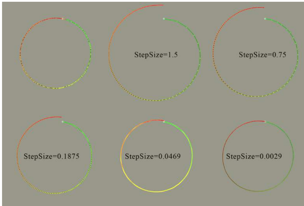
Figure 7.5: Comparison of the integration methods Euler and Dop853. A correct integration should yield a circle, like, when using Dop853 (top left). An Euler integration with the same number of steps results in a spiral shape (top mid). Decreasing the step size of the Euler integration finally yields a circle but with a higher computation time than Dop853 (top right via bottom left to bottom right). Data according to the illustration is gather in the table.
